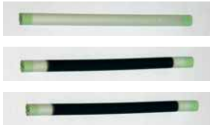
Co-sintered NiO-YSZ/YSZ and NiO-YSZ/YSZ/LSM tubular anode supports, Photo: ARC Austrian Research Centers GmbH
